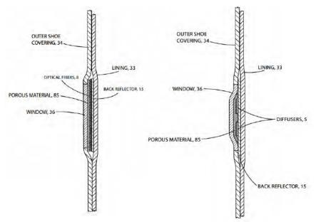
According to Stride Rite, the use of discrete LEDs (denoted as "Diffusers, 5" in the above illustration) would create space between the light sources in which the back reflector (i.e. the interfacing layer) would be "adjacently connected" to the light diffusing layer. In support of its proposed modification, Stride Rite cited to the declaration of Holden, who opined that replacing the optical fibers of Parker with Rosko's LEDs would "increase the durability
