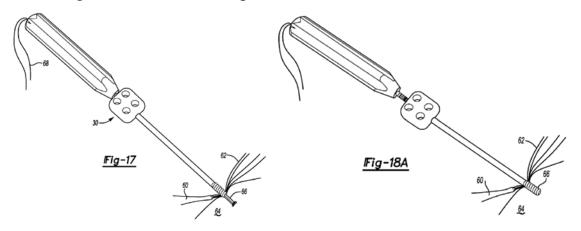
Figures 17 and 18A illustrate the driver, screw and suture loop engaging graft sutures in a bone socket. *Id.* at 2:52–57.
