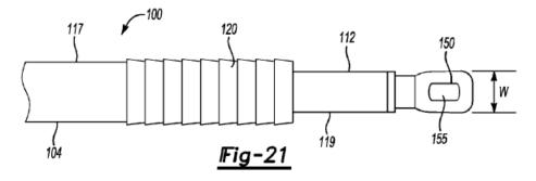
Figure 21 depicts driver 100, interference device 120, and eyelet implant 150. *Id.* at 6:47–55, 7:4–5.
