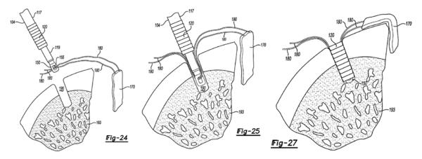
Figures 24, 25, and 27 are schematic views of the surgical site undergoing a graft fixation with a push lock driver. *Id.* at 3:8–23.
