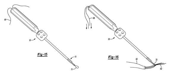
Figures 15 and 16 illustrate a driver, screw, suture loop and graft with graft sutures attached. *Id.* at 2:46–50.
