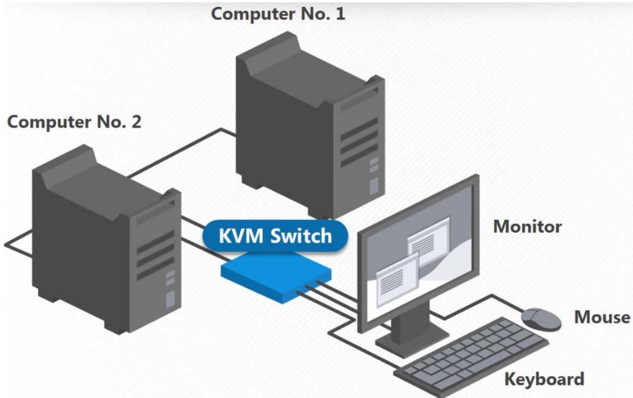
A KVMP—keyboard, video, mouse, peripheral—switch provides a slight variation on this. As its name suggests, a KVMP switch adds a peripheral, like a printer or scanner, to the mix. A user of one computer with a printer can switch to another computer using a KVMP switch, and choose to have the printer follow to the second computer or remain with the first computer.
