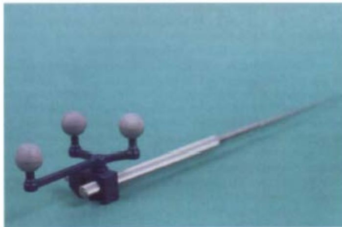
Fig. 3. Passive-marker arrays were developed that can easily be attached to any already existing surgical instrument. Thus any instrument can be used as a navigation tool merely by simple calibration of its geometry. This saves cost and frees the surgeon from the restriction of using special pointers.
