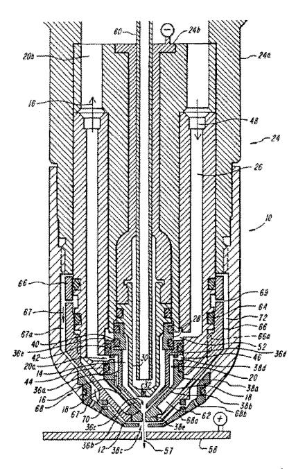
The torch 10 as depicted in Figure 5 includes a body 24 supporting an electrode 30 and a two piece nozzle 34 (not enumerated; see Fig. 7). (Couch '126, col. 4, ll. 17–24; see also Fig. 7).
