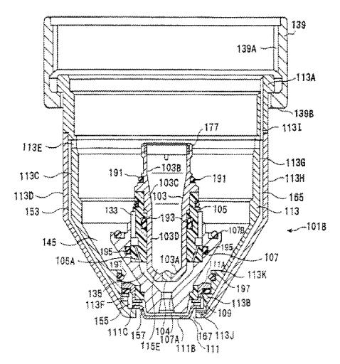
The detachable unit as depicted in Figure 3 includes an electrode 103, an insulating guide 105 and a nozzle 107 received inside a retainer cap 113. (See '156 patent, col. 16, ll. 17–19). An internally threaded rotating ring 139 couples the retainer cap 113 to the torch main unit 101A. (See '156 patent, col. 12, ll. 20–37; & Figs. 1 & 3).
