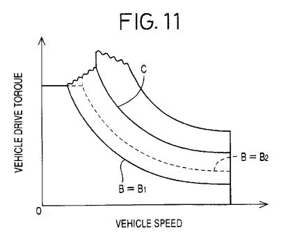
Figure 11 shows a graph which represents a predetermined relationship between the vehicle drive torque and running speed.
