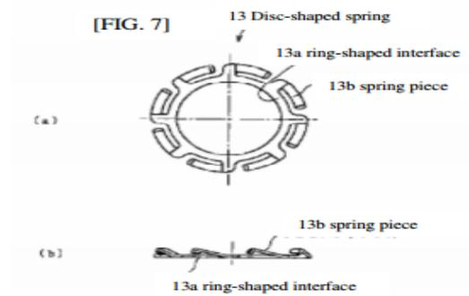
As shown in Figures 7(a) and 7(b) of Tatsuzuki, disc-shaped spring 13 is formed by stamp cutout processing of a thin metal plate possessing elasticity, e.g., phosphor bronze. Ex. 1002 ¶ 17. Disc-shaped spring 13 includes spring piece 13b and ring-shaped joining part 13a. *Id.* Spring piece 13b includes eight bent spring pieces, which are formed integrally by ring-shaped joining part 13a. *Id.*
