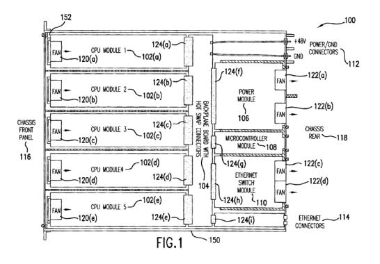
Figure 1 is a schematic illustration of a computer network appliance. As shown above in Figure 1 of the '021 patent, computer network appliance 100 includes CPU modules 102(a)–(e), power module 106, microcontroller module 108, and Ethernet switch module 110 connected to the backplane 104 via hot swap connectors. *Id.* at 3:18–23, 32–37.
