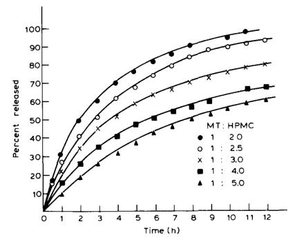
Fig. 2. Release of metoprolol tartrate (cumulative percent) as a function of time from tablets containing drug: HPMC in the ratios given.
