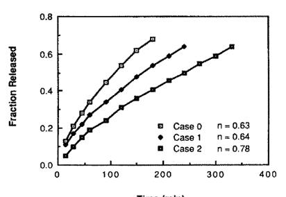
Time (min) Fig. 5. Drug release profiles of the systems. Calculated values of exponent n of Eqn 2 are also shown.
