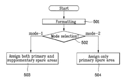
Figure 5 illustrates a flow chart showing a method of assigning the spare area(s) of an optical recording medium. According to the disclosed
