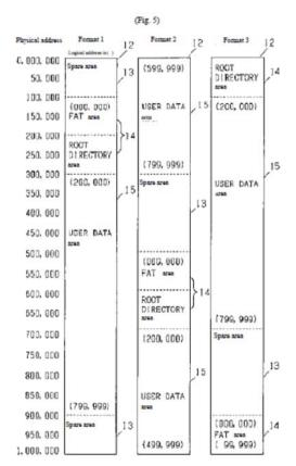
Figure 5 of Kawano above shows three format arrangements with spare areas 13. *See id.* ¶ 16. As illustrated in Kawano's Figure 5, "[i]n format 1, the two spare areas 13 are 0 - 99,999 and 9,000,00 - 1,000,000" and "in format 2, . . . the spare area is started from 300,000." *Id.*.
