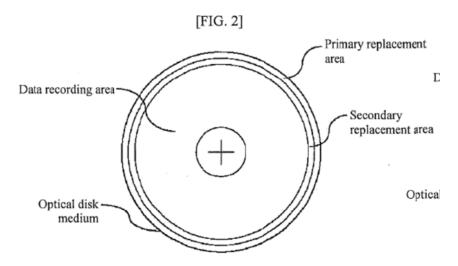
Ohata's Figure 2 shows a data recording area, a primary replacement area, and a secondary replacement area in a disc.
