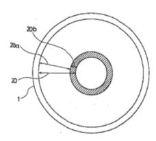
Figure 5 shows an example of alternative tracks 20b in a conventional magnetic disc. *See* Ex.  $1007 \, \P \, 6$ . According to Ozaki, "alternative track 20b is disposed at several tracks of the innermost circumference with respect to a normal usage area 20a among the total usable track area 20 on a magnetic recording medium 1." *Id*.
