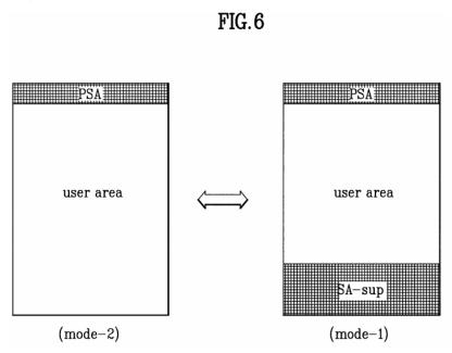
Figure 6 illustrates examples of first and second modes of assigning spare areas during formatting. As depicted, the size of the PSA in each mode is equal, providing a stated benefit of allowing convenient mode conversion. *See* Ex. 1001, col. 2, ll. 47–54, col. 3, ll. 15–43. As the arrow in Figure 6 signifies, "the present invention allows a conversion between the
