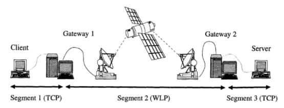
Figure 1 depicts a communication system divided into three segments, with a wired communication connection from a Client computer to Gateway 1, a wireless connection from Gateway 1 to Gateway 2, and a wired connection from Gateway 2 to a Server. *Id*.
