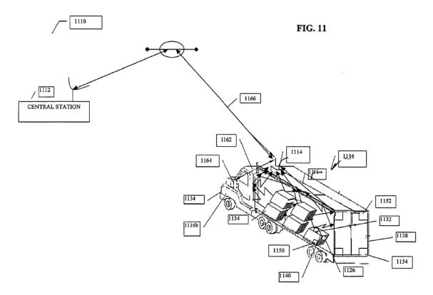
*Id.* at Fig. 11. Figure 11 shows an "asset, object, people or animal monitor 1114," which is associated with a truck carrying cargo 1134. *Id.* ¶ 128, Fig. 11. Cargo 1134 may be "large items such as a refrigerator or a number of smaller items on a pallet or in a crate." *Id.* ¶ 129. Sensors 1126 are attached to cargo 1134 to monitor its status (e.g., temperature) and report to monitor
