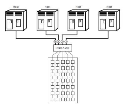
Figure 1-2 of the CRD Manual depicts a configuration of the CRD-5500 controller where each of four different hosts is assigned to a different channel, i.e., channel 0 through channel 3. Ex. 1004, 10. These hosts may then access redundancy groups via the CRD-5500 controller. *Id*.
