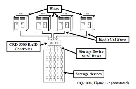
Figure 1-2 shows the architecture of a network using the CRD-5500 with hosts attached to SCSI buses on one side of the controller and storage devices also attached to SCSI buses on the other side. *Id.* at 10–13.
