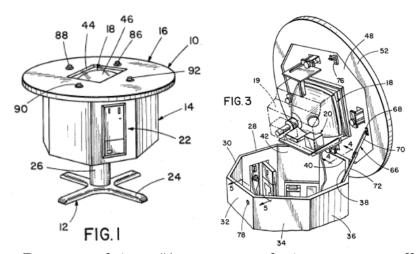
As Runte explains: "Amusement device 10 generally consists of a support 12, a housing 14 mounted on the support 12, a table top 16 hingedly mounted on the housing 14, [and] a conventional cathode ray tube 18 mounted on the interior of table top  $16 \dots$ " *Id.* at col. 2 ll. 41–45.
