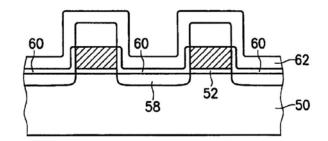
*id.* fig. 2B; *see also id.* fig. 1B. Later, a portion of the thin oxide layer is removed "to expose the diffusion region." *Id.* col. 1 ll. 38–40, col. 3 ll. 22–24.
