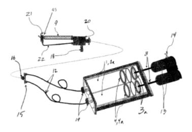
The claimed device includes, inter alia, two cylindrical cartridges (1, 1a), a static mixing nozzle (9), a spray tip (21), and first and second flexible tubes (12). The apparatus permits the simultaneous mixing, dispensing, and spraying of two-component paints in industrial settings.
