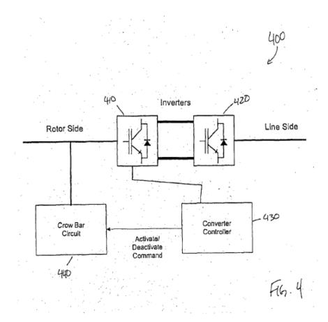
Figure 4 shows back-to-back inverters as part of the power converter; the inverters receive power as needed during a low voltage event "to keep the wind turbine generator connected to and synchronized with the power grid." '985 patent, col.6 ll.27-29. The specification describes the connections and functions of the components, including the following:
