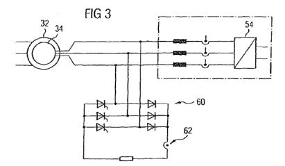
The specification explains that the crowbar circuit 60 is deactivated, the bridge is blocked, and the rotor windings are recoupled, when the current drops to the predetermined value.
