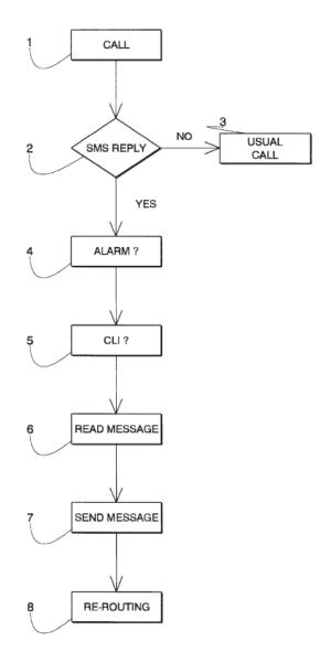
Mäkelä's Figure 1 "illustrates as a simple flow diagram a preferable embodiment of the method in accordance with the method." *Id.* at 4:56–57. Step 6—which is performed after the call is received—shows that the message is read from memory and sent; but there is no teaching or
