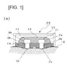
Figure 1(a) depicts pulse wave sensor 20 including light emitting device 21 and light receiving device 22, which are enclosed and supported by sensor case 23 and shell supporting member 29. *Id.* ¶ 9. Sensor 20 also includes light guide 21b extending from light emitting device 21 to direct infrared light to wrist 10 and light guide 22b extending to light receiving device 22 to
