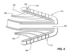
Figure 4 depicts a section of first end 112 of conductor portion 104. *Id*. ¶¶ 22, 33. Fiber optic cables 402 terminate in optically transparent elastomer 408 of first end 112 to allow the communication of light between fiber optic cable 402 and the tissue of the auditory canal wall. *Id*. ¶ 33.
