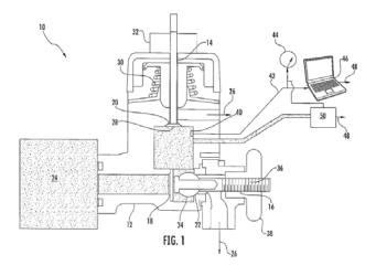
J.A. 48–52, 60. The '222 application explains that the sensor generates a "signal" 42 reflective of the fluid pressure in the chamber between the valves and transmits the signal to an indicator 44, such as a pressure gauge. J.A. 51. The signal can then be compared to a predetermined limit to generate a control signal, which, in turn, can be used to control or adjust one or more of the two valves to drain fluid as appropriate. J.A. 51–52.
