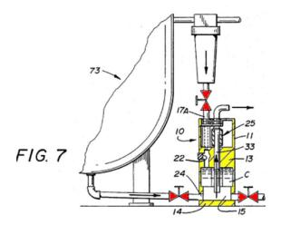
Appellant's Br. 22 (citing Rasmussen fig.7 (annotated)); see also Appellee's Br. 5 (annotating Rasmussen's Figure 7 to point to the same valve); J.A. 118 (examiner's rejection pointing to the same valve). As shown, the unlabeled valve—and, therefore, the inlet seat therein<sup>4</sup>—
