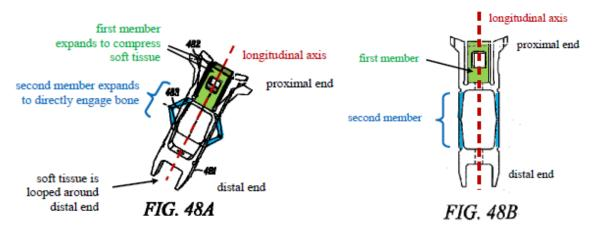
Figures 48A and 48B illustrate isometric and side views of a substantially non-cylindrical multiple component tendon anchor with two levels of expanding sections, as an embodiment of the '294 patent. Ex. 1001, 7:49–52. According to Patent Owner:
