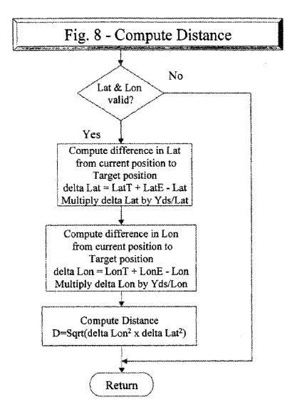
Figure 8 not only discloses the formula for computing the distance between a current position and a target object, but it includes "LatE" and "LonE" as terms in the algorithm. "LatE" is the "eFilter Lat [latitude] correction value," and "LonE is the "eFilter Lon [longitude] correction value" (col. 11, 11. 36-37). Figure 8 therefore further suggests that eFilter environmental error correction forms part of the distance determining process.
