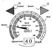
Thus, Nagoshi discloses adjusting a colored display, namely the green and red LEDs, in response to the speed limit at the vehicle's present location. Garmin
