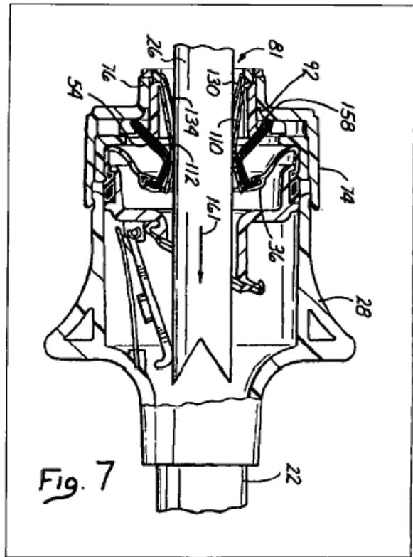
These figures disclose an embodiment of the claimed trocar both with (Figure 7) and without (Figure 6) an instrument 26 inserted through orifice 38. The parties refer to this structure as the “ring-levers-teeth” embodiment. In this embodiment, the septum
