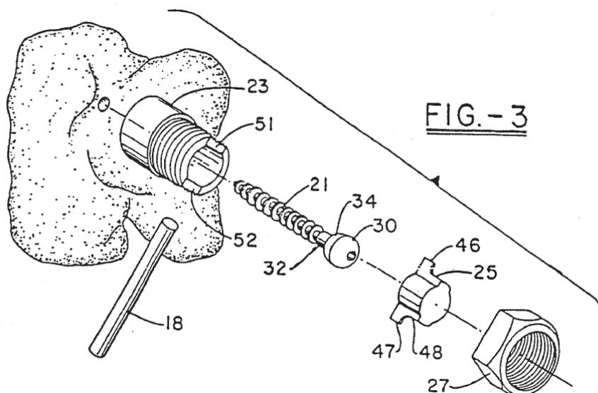
On appeal, this court identified the function of the securing means as “caus[ing] the rod [18] to bear against the rod-receiving channel [51-52] by applying a compressive force in the direction of the vertical axis while ensuring that substantially equal forces are applied along the longitudinal axis of the rod [18] on opposite sides—either inside or
