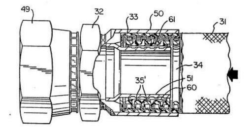
Ridges and recesses circumscribe the interior corrugated surface of the hose. The coupling includes an outer sleeve (50) having a flat inner surface and an inner sleeve (51) having a contoured outer surface, the sleeves respectively contact the exterior and interior surfaces of the hose (31). The inner sleeve, the contours on the outer surface of which complement the ridges and recesses of the hose, is expanded outwards to seal the hose between the outer sleeve and the inner sleeve.
