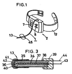
Applying its construction of "electrochemical sensor" as covering sensors with external cables or wires, the
