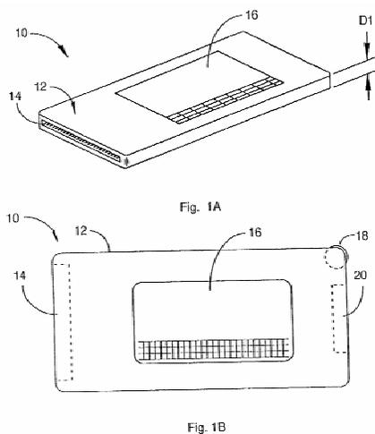
As shown in the drawings, the PDA includes a thumbwheel controller (18), a user interface (16), a host interface (14) for connection to the host computer, and a second external connector (20) for connection to external devices such as printers. The patent explains that
