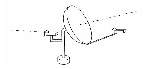
According to Northpoint, the terrestrial signal will not interfere with the DBS signal or vice versa because the terrestrial signal will be transmitted in a specific azimuth spaced away from the DBS satellite-to-user azimuth. Northpoint claims that in such a case, the signal received by each antenna at the user location will be outside the "directional reception range" of the other antenna. Claim 8 of the '605 patent provides as follows:
