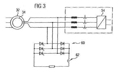
The specification explains that the crowbar circuit 60 is deactivated, the bridge is blocked, and the rotor windings are recoupled, when the current drops to the predetermined value.
