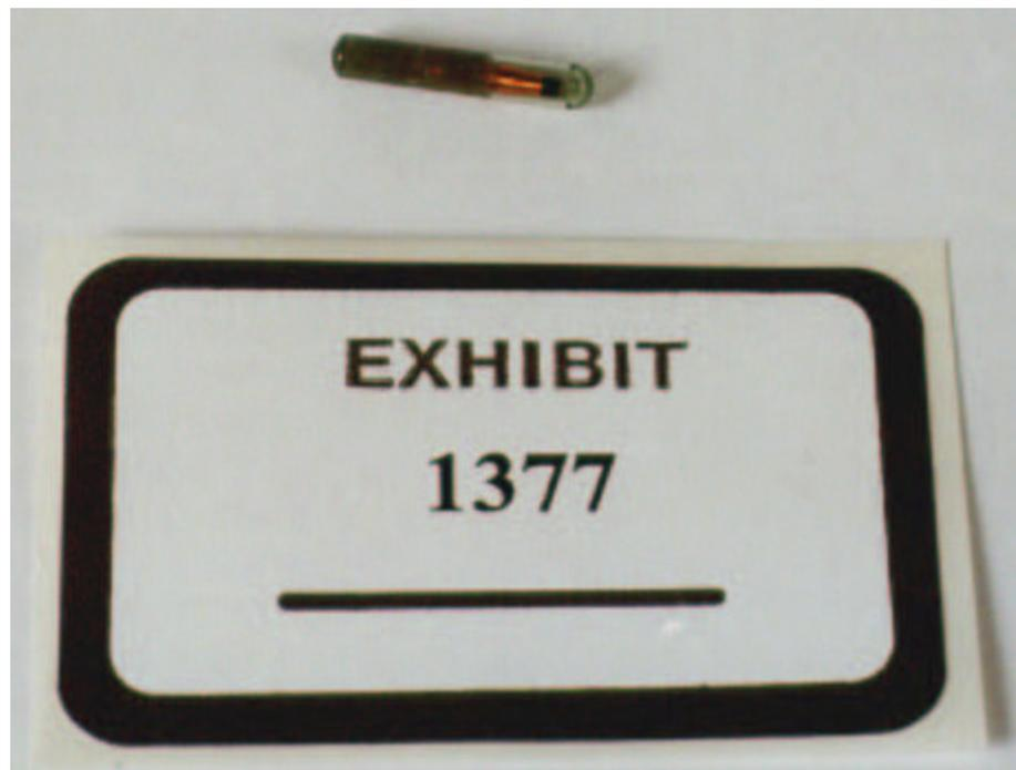
Passive transponders are generally affixed to objects that require identification. To read the identifying information contained in a transponder, an external reader transmits an electromagnetic signal that is received by the transponder antenna. The signal generates electrical energy in the antenna coil which activates the integrated
