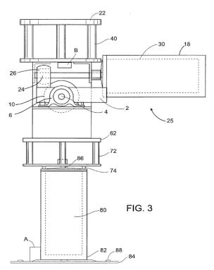
The '662 patent further teaches a method to achieve a third axis of stabilization along the azimuth axis. Fig. 3 compensates for azimuth motion by adding a third set of orthogonally positioned drive components to the stabilized platform 100. This third drive mechanism stabilizes the platform with input from sensor packages A and B. Sensor package A appears on the housing 82, or other disclosed areas; package B on the camera platform 22. *Id.* at col. 5 ll. 26-39; col. 4 ll. 25-27.
