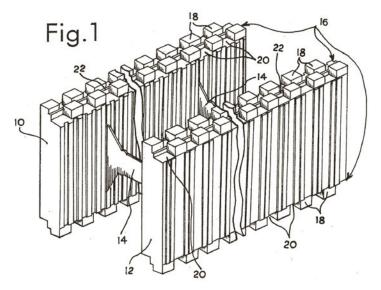
The specification explains that, unlike prior art ICFs, which had to be arranged in a specific way for interconnection, the claimed ICFs are designed to permit interconnection "with like blocks or panels in a bi-directional and/or reversible manner." '933 Patent, col. 1, ll. 8-13.
